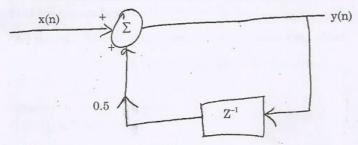
Find the frequency response H(eim) and the impulse response h(n) of the system. Sketch the magnitude response | H(e<sup>j\omega</sup>) | for the system.
